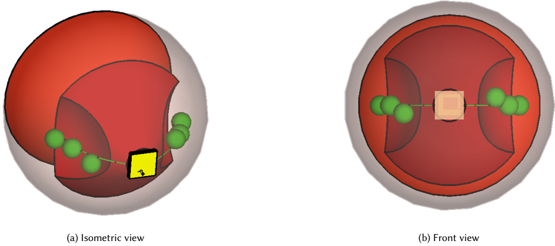
Fig. 4. 3D views of breast phantom with mounted antenna
